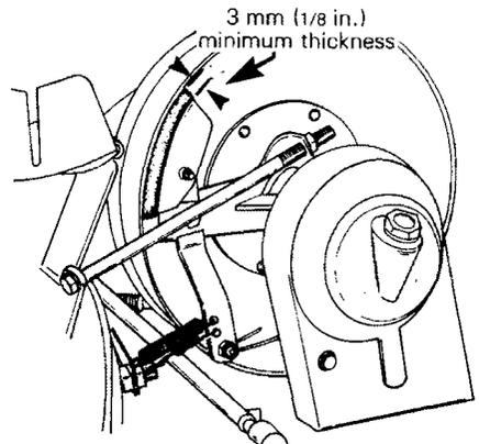
◆ **WARNING:** Brake pad or puck less than 3 mm (1/8 in.) thick must be replaced. Replacement must be performed by an authorized dealer.
