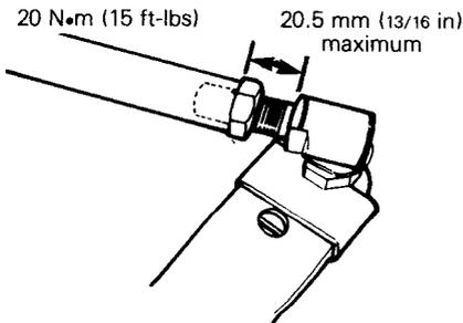
Handlebar should also be horizontal when the skis are pointed toward the front. To adjust; loosen the lock nuts of the shorter tie rod. Turn the tie rod manually until the handlebar is horizontal. Retighten the lock nuts firmly. Check tightness of the steering arm locking bolts and the wear of the ball joints.
