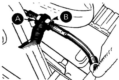
Once minor adjustment is completed, firmly tighten the nuts (A and B) against the bracket. If correct brake control lever clearance is unobtainable, proceed with major adjustment as follows:
