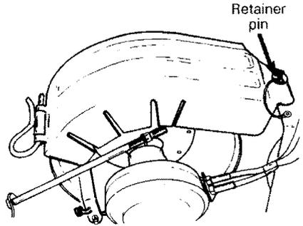
3. To remove the drive pulley guard, pull out the retaining clip (A) and pull on the spring (B) to disengage the pin from the bracket.
