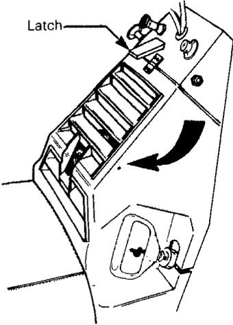
2. Push the console downward then tilt away from the engine. To re-install, reverse the procedure.
