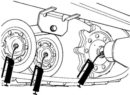
▼ **CAUTION:** Always use a low pressure grease gun when lubricating rear axle.
