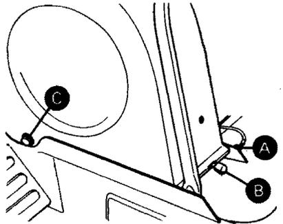
4. Push the pulley guard forward to disengage the front attachment (C) from the frame. Lift the guard from the vehicle.
