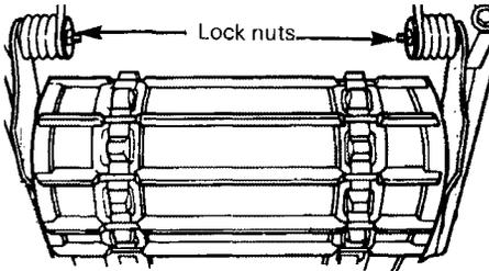
2. Adjust to proper tension by turning adjuster bolts clockwise to tighten counter-clockwise to slacken. Adjust both sides equally.
