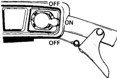
◆ **WARNING:** For safety reasons, the emergency cut-off switch is easily accessible; be careful not to operate it inadvertently.
