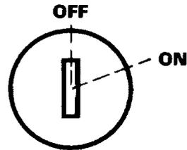
Key operated, 2 position switch. To start the engine, first turn the key clockwise to ON position. To stop the engine, turn the key counter-clockwise to OFF position.
