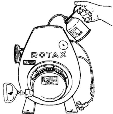
Slowly crank the engine several times using the manual starter.
