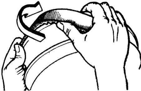
4. Slip the belt out from the drive pulley and remove completely from the vehicle. To install the drive belt, reverse the procedure.
