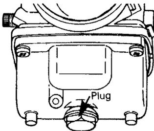
Reinstall the plug and connect the fuel line.
