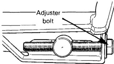
○ **NOTE:** Track tension and alignment are inter-related. Do not adjust one without checking the other.
