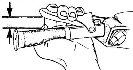
If a minor adjustment is indicated, slack off the cable housing nut (A) and tighten the nut (B) to increase the lever clearance.
